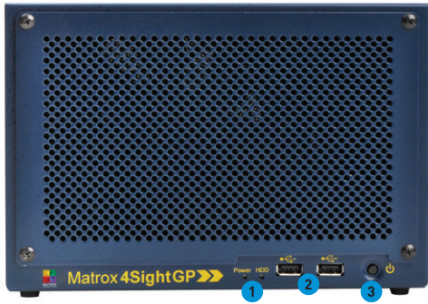
1. Status LEDs 2. USB 2.0 ports 3. Power switch
