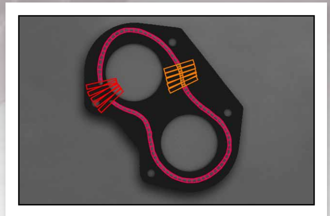
MIL Bead Inspection
